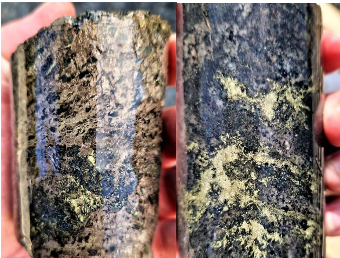
Figure 1: Vuostok Project – Drillhole VUO23012, clusters of massive sulphides showing nickel-copper sulphides (pyrrhotite, pentlandite and chalcopyrite)
